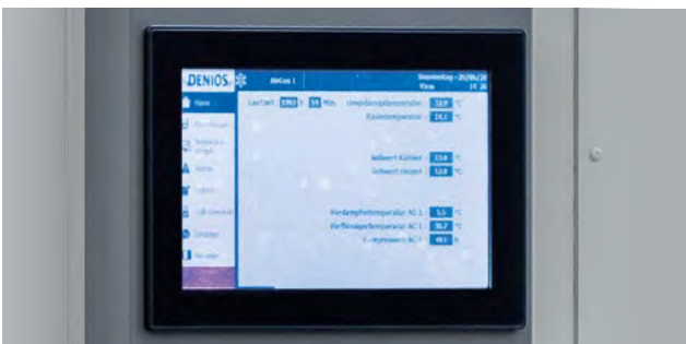
Central monitoring and control of all electrical components with the Communication Bar
